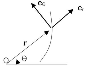
$\Sigma F_r = m a_r = m (\ddot{r} - r\dot{\theta}^2), \quad \Sigma F_\theta = m a_\theta = m (r\ddot{\theta} + 2\dot{r}\dot{\theta})$
