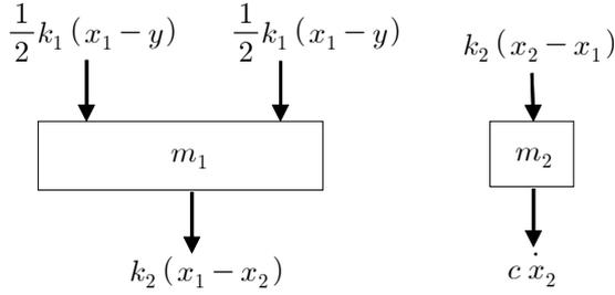
$$\begin{aligned} \text{(b)} \quad m_1 \ddot{x}_1 &= -k_1(x_1 - y) - k_2(x_1 - x_2) & \Rightarrow & \quad m_1 \ddot{x}_1 + (k_1 + k_2)x_1 - k_2x_2 = k_1 y(t) \\ m_2 \ddot{x}_2 &= -k_2(x_2 - x_1) - c \dot{x}_2 & \Rightarrow & \quad m_2 \ddot{x}_2 + c \dot{x}_2 - k_2x_1 + k_2x_2 = 0 \end{aligned}$$
