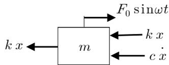
$$-kx - kx - c\dot{x} + F_0 \sin\omega t = m\ddot{x}$$
