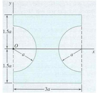
$$\begin{aligned} I_{y1} &= \frac{1}{3}b^3h = \frac{1}{3}(3a)^3(3a) = 27a^4 = 27 (20 \text{ mm})^4 \\ &= 4,320,000 \text{ mm}^4 = 4,320 \times 10^3 \text{ mm}^4 \end{aligned}$$
