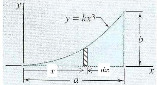
$$9.4 \quad dI_y = x^2 dA = x^2 y dx = x^2 \frac{b}{a^3} x^3 dx = \frac{b}{a^3} x^5 dx$$
