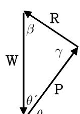
$$\frac{P}{\sin\beta} = \frac{W}{\sin\gamma} \Rightarrow P = W \frac{\sin\beta}{\sin\gamma} = (600 \text{ N}) \frac{\sin 46.31^\circ}{\sin 103.69^\circ} = 446.5 \text{ N} \Rightarrow P = 447 \text{ N}$$
