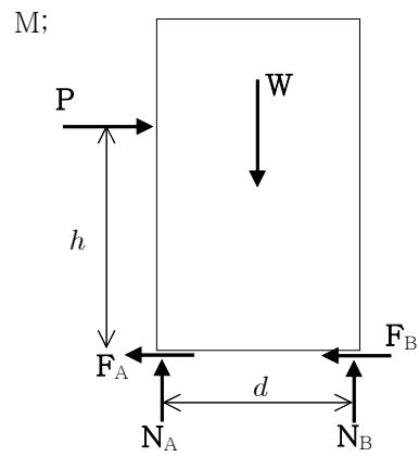
$$8.9 \quad W = 600 \text{ N}, \quad \alpha = 35^\circ, \quad \mu_s = 0.25, \quad \mu_k = 0.20, \quad \theta = 60^\circ$$
