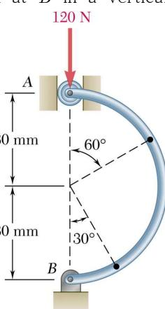
(b) Determine the horizontal and vertical components of the reaction at *B*.
