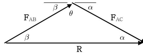
$F_{AB} = 2.2 \text{ kN}$ ,  $\alpha = 25^\circ$ ,  $\beta = 30^\circ$ ,  $R$  is horizontal. (a)  $F_{AC} = ?$ , (b)  $R = ?$
