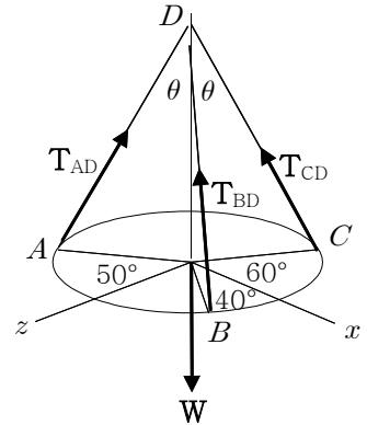
$$(T_{CD})_y = T_{CD} \cos\theta, \quad (T_{CD})_h = T_{CD} \sin\theta$$
