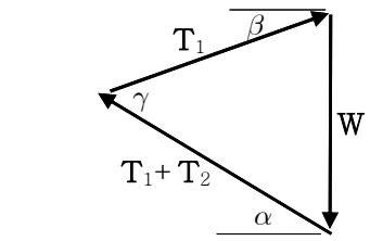
$$(b) \frac{T_1 + T_2}{\sin(90^\circ - \beta)} = \frac{W}{\sin\gamma}$$
