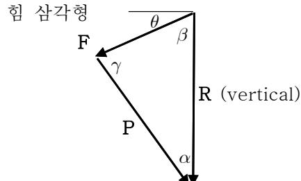
$$F = 1600 \text{ N}, \quad \theta = 15^\circ, \quad \alpha = 25^\circ$$
