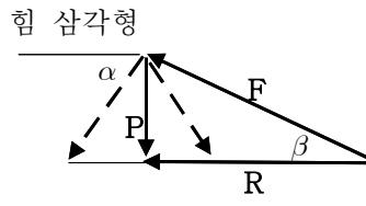
$$F = 50 \text{ N}, \quad \beta = 25^\circ, \quad P \text{가 최소이려면 } \alpha = 90^\circ$$
