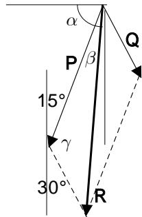
$$P = 45 \text{ N}, \quad Q = 15 \text{ N}, \quad \gamma = 180^\circ - (15^\circ + 30^\circ) = 135^\circ$$
