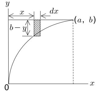
$$\begin{aligned} I_y &= \int dI_y = \int_0^a \frac{b}{a^2}(x^4 - 2ax^3 + a^2x^2) dx \\ &= \frac{b}{a^2} \left[ \frac{1}{5}x^5 - \frac{a}{2}x^4 + \frac{a^2}{3}x^3 \right]_0^a = ba^3 \left( \frac{1}{5} - \frac{1}{2} + \frac{1}{3} \right) = \frac{a^3 b}{30} \end{aligned} \quad ( )$$
