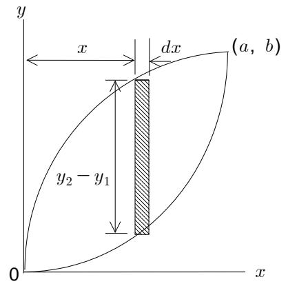
$$dI_y = x^2 dA = x^2 \left( \frac{b}{a^{1/4}} x^{1/4} - \frac{b}{a^4} x^4 \right) dx = \left( \frac{b}{a^{1/4}} x^{9/4} - \frac{b}{a^4} x^6 \right) dx$$
