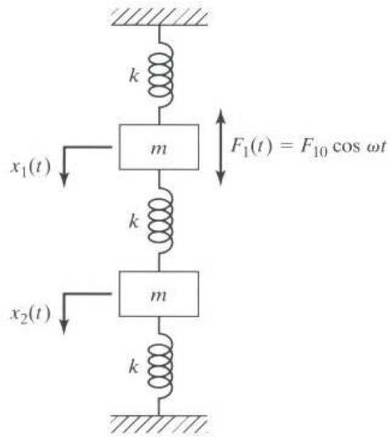
**FIGURE 5.15** A two-mass system subjected to harmonic force.
