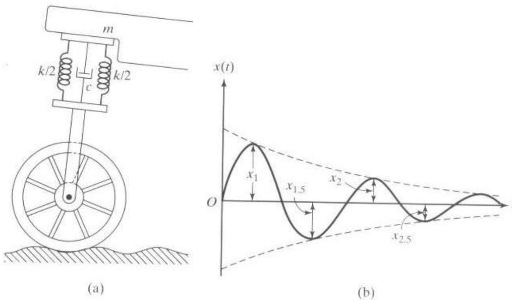
FIGURE 2.30 Shock absorber of a motorcycle.
